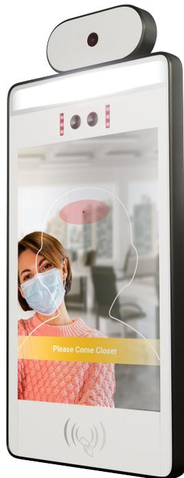
As you approach the device, fill the silhouette with your face/head but do NOT exceed the shape. Leaning in/out helps while maintaining the 20" distance.
