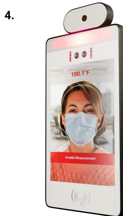
If the device measures your temperature above the set threshold, red lights will flash, alarm will sound, and you will hear:
